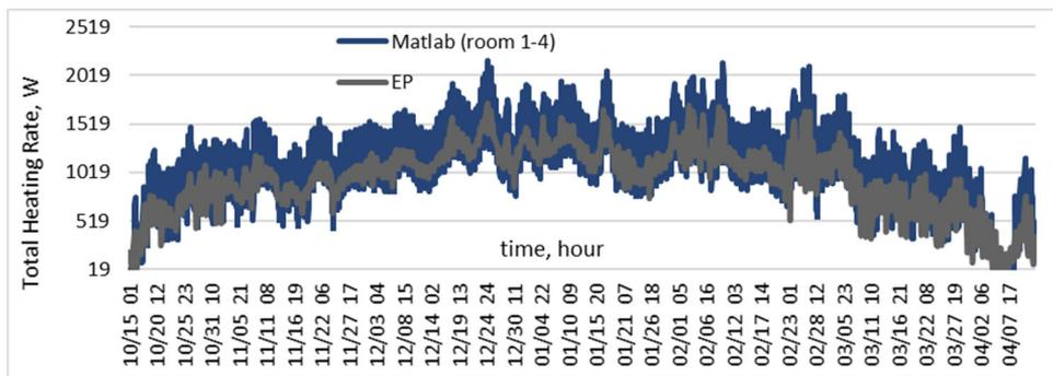
**Fig. 6.** The load on the heating system of the apartment for the heating season
