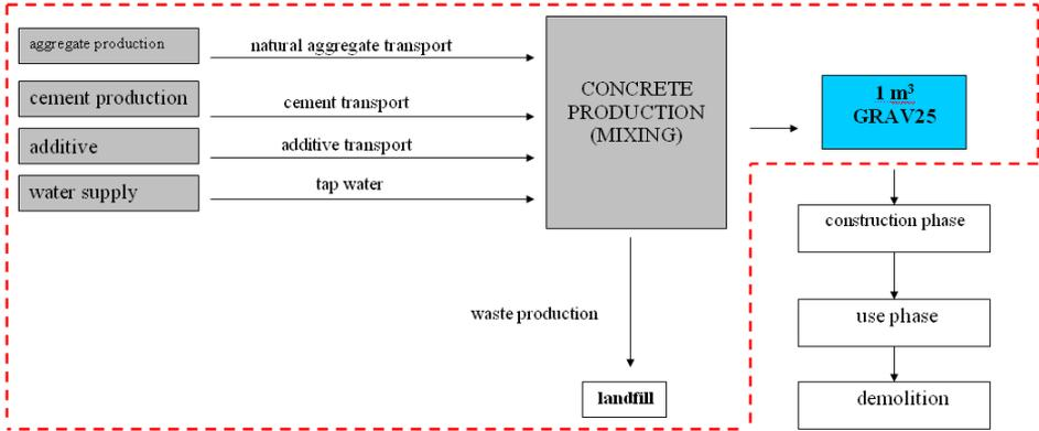
**Fig. 2.** System boundaries, processes and materials for conventional concrete production system
