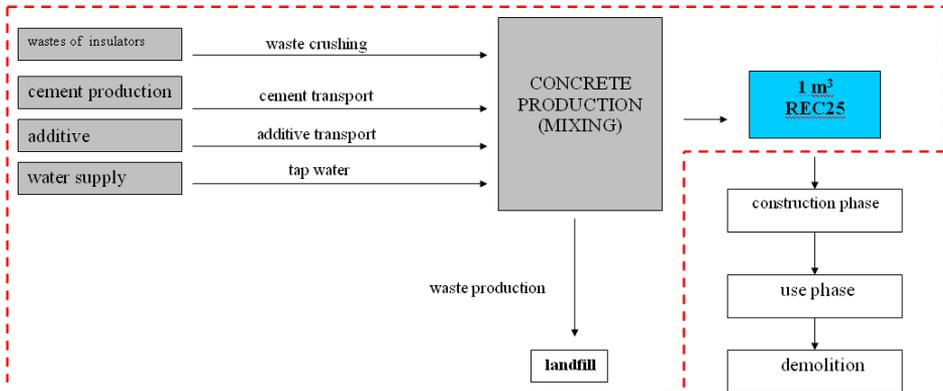
**Fig. 3.** System boundaries, processes and materials for recycled concrete production system
