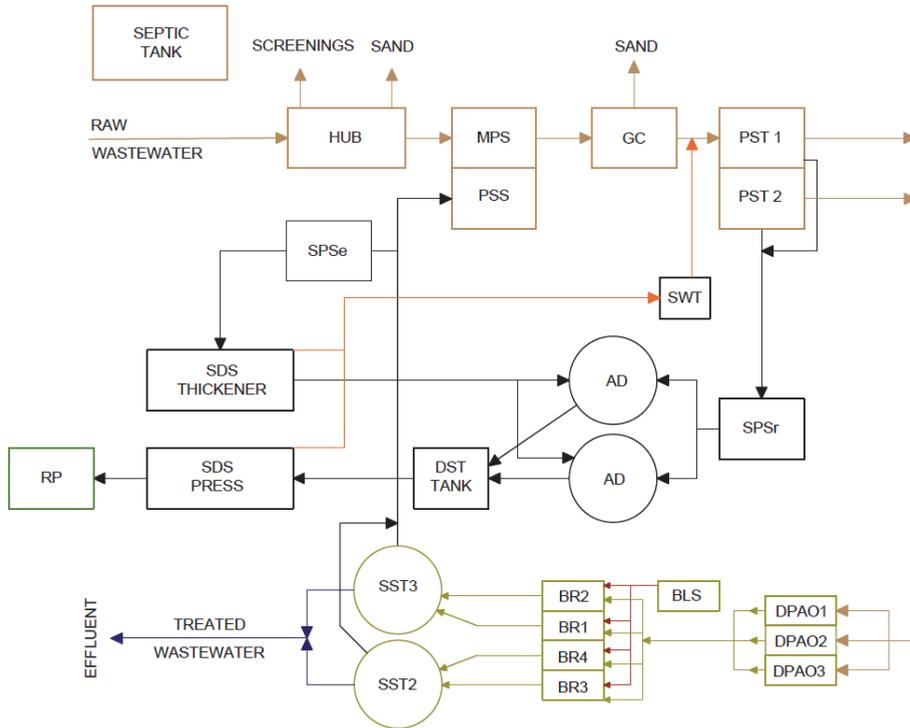
**Fig. 1.** Block diagram of the wastewater treatment plant in Żory. Source (Own materials of PWiK Żory 2018; Zdebek et al. 2018)
