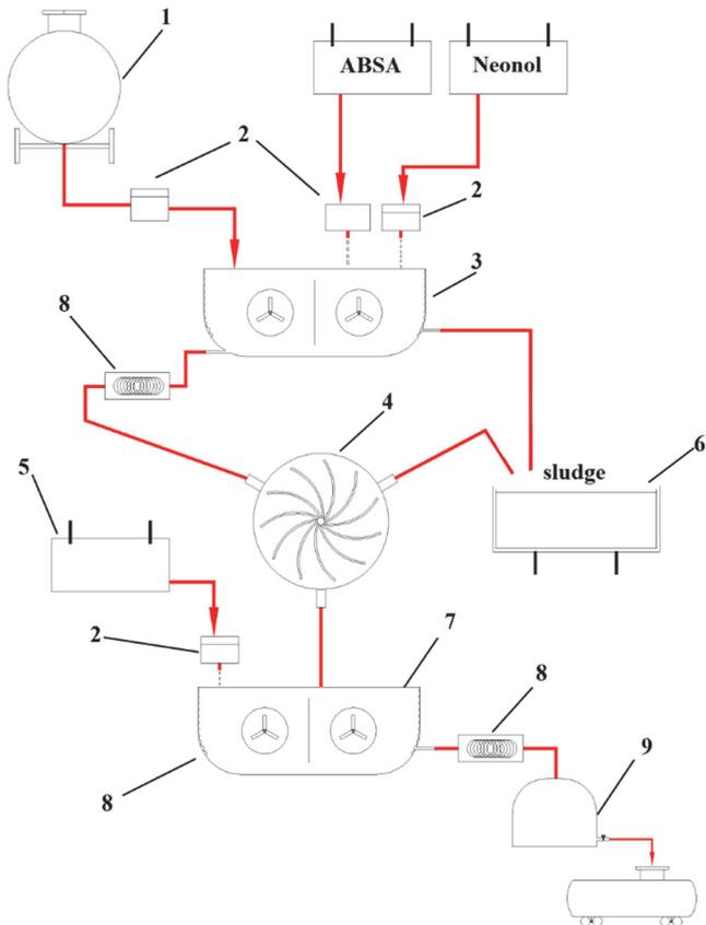
**Fig. 1.** Scheme for treatment of discarded waste oil; 1 – balance tank, 2 – dosing pumps, 3 – first-stage mixer with heating, 4 – centrifuge, 5 – additive storage tank, 6 – sludge collector, 7 – second-stage mixer, 8 – pumps, 9 – storage tank for restored oil
