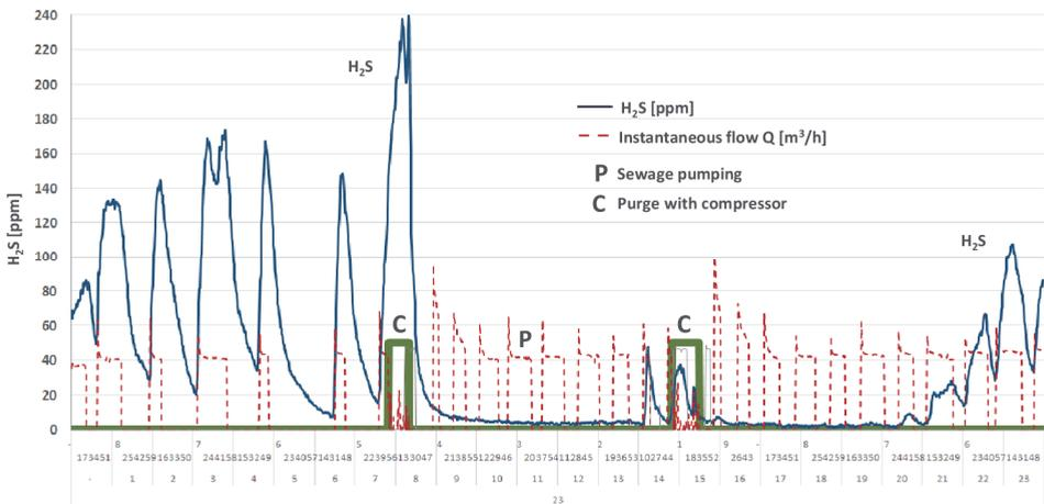
**Fig. 5.** Daily changes in hydrogen sulfide concentration for two exemplary purges in the EST system during the day (23.08.2019) at Object-2
